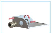
1. Install cable gland to the enclosure with the indicated "torque body". In order to increase contact quality EMC locknut utilization is recommended.
