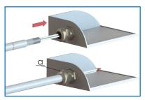
**3.** Insert cable Into cable gland until marking "a" aligns with cap. EMC component will contact shielding.
