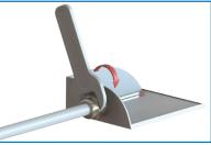
**5.** Tighten cap and apply indicated "torque cap".
