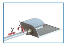
4. Do not pull or rotate cable after insertion. In doing so cable gland and shielding will be damaged.
