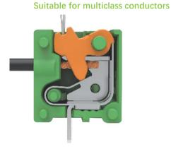
Depressing the button releases the wire and reset spring to its initially open state, ready for the next wiring.
