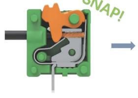
As soon as the wire comes into contact with the spring, the spring is triggered and the wire is clamped. A clear "click" sounded, indicating that the connection is complete!
