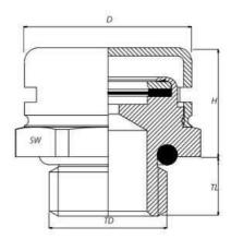
In order to choose the right ventilation plug unit (pressure balance elements) for a specific application, the working principles of the unit must be known first Ventilation plugs are permeable to "gases and vapours, e.g. air" but impermeable to "liquids and dust, e.g. water". The permeability resistance to liquids depends on the pore size and structure of the membrane inside these devices.
