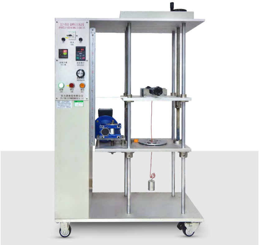
Din Rail Terminal Blocks Rotational Pull Test
