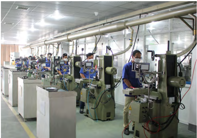
High precision surface grinding machines (30 sets)
