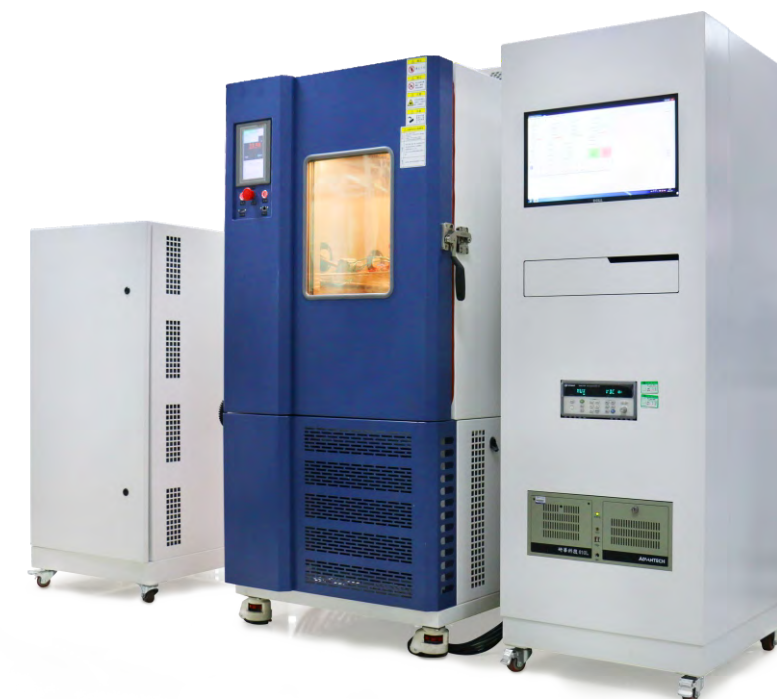
Screwless Terminal Blocks Temperature Cyclic Aging Test System
